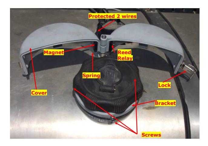
The plastic Fuel Cap Protector is mounted on the fuel lid using the bracket and three Allen screws. A lock is used to close the two parts of the cover. The spring enables automatic opening of the cover when the lock is opened. When the cover is closed, the reed relay is adjacent to the magnet and the two wires are connected to each other. When the cover is opened the reed relay opens the circuit and disconnects the two wires.
